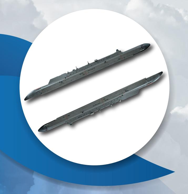
LM52M2 / LM52AS Launcher provides for a locked flight, preparation and firing of MAGIC 2 auto guided infrared missile. It equips MiG 21 Lancer aircrafts.
